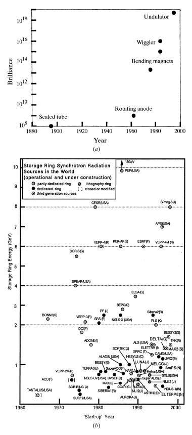
Fig. 8.1.2.1. (a) Evolution of X-ray source brilliance (photons s<sup>-1</sup> mrad<sup>-2</sup> mm<sup>-2</sup> per 0.1%  $\delta\lambda/\lambda$ ) in the hundred years since Rontgen's discovery of X-rays in 1895. Adapted from Coppens (1992). (b) The evolution of storage-ring synchrotron-radiation sources over the decades, as illustrated by their increasing number and range of machine energies up to the present (Suller, 1998).
