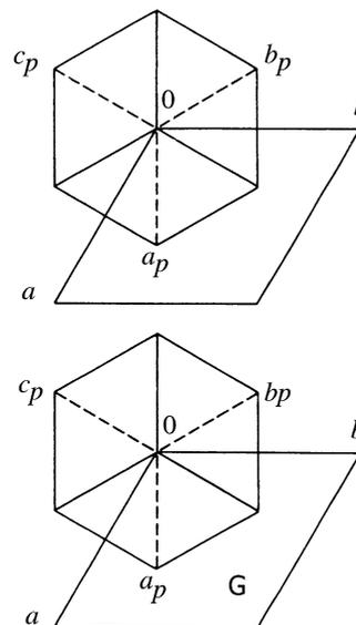
Fig. 2.2.6.9. Rhombohedral *R* space groups. Obverse triple hexagonal cell with ‘hexagonal axes’ *a*, *b* and primitive rhombohedral cell with projections of ‘rhombohedral axes’ *a<sub>p</sub>*, *b<sub>p</sub>*, *c<sub>p</sub>*. Note: In the actual space-group diagrams only the upper edges (full lines), not the lower edges (dashed lines) of the primitive rhombohedral cell are shown (G = general-position diagram).
