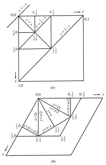
Fig. 2.2.8.1. Boundary planes of asymmetric units occurring in the spacegroup tables. (a) Tetragonal system. (b) Trigonal and hexagonal systems. The point coordinates refer to the vertices in the plane z = 0.
