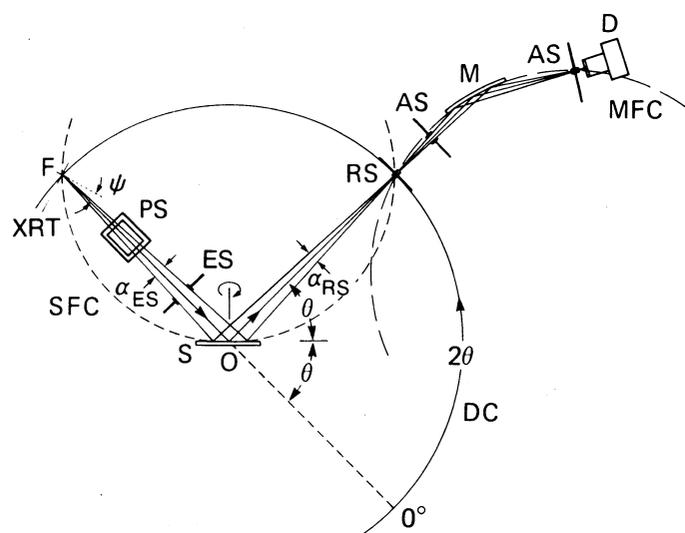
Fig. 2.3.1.3. X-ray optics in the focusing plane of a 'conventional' diffractometer with reflection specimen, diffracted-beam monochromator, and  $\theta$ - $2\theta$  scanning:  $\psi$  take-off angle, DC diffractometer circle, MFC monochromator focusing circle,  $\alpha_{ES}$  and  $\alpha_{RS}$  entrance- and receiving-slit apertures,  $\theta$  Bragg angle,  $2\theta$  reflection angle,  $O$  diffractometer and specimen rotation axis; other symbols listed in Fig. 2.3.1.1.
