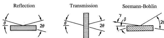
Fig. 2.3.1.2. Specimen orientation for three diffractometer geometries. With  $\theta$ - $2\theta$  scanning, diffraction is possible only from planes nearly parallel to the reflection specimen surface (left), and from planes nearly normal to the transmission specimen surface (middle), and from planes inclined different amounts to the specimen surface in Seemann-Bohlin geometry (right).
