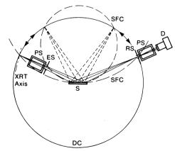
Fig. 2.3.1.14. Optics of  $\theta$ - $\theta$  scanning diffractometer. X-ray tube and detector move synchronously in opposite directions (arrows) around fixed horizontal specimen. A focusing monochromator can be used after the receiving slit.
