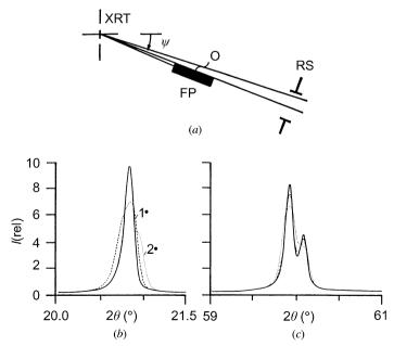
Fig. 2.3.1.7. (a)  $\theta$ -2 $\theta$  setting at 0°. Flat plate or long narrow slit is rotated to position of highest intensity. (b) and (c) Profiles obtained with correct  $\theta$ -2 $\theta$  setting (solid profile) and 1 and 2° mis-settings (dashed profiles) at (b) 21° and (c) 60° (2 $\theta$ ).
