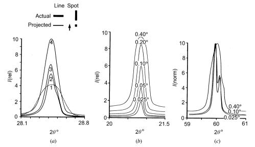
Fig. 2.3.1.9. (a) Effect of source size on profile shape, Cu  $K\alpha$ ,  $\alpha_{\rm ES}$  1°,  $\alpha_{\rm RS}$  0.05°, Si(111).
