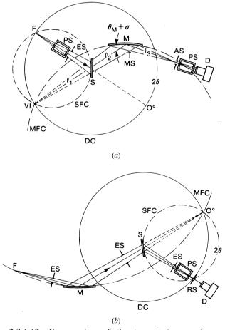
Fig. 2.3.1.12. X-ray optics of the transmission specimen with asymmetric focusing monochromator and  $\theta$ -2 $\theta$  scanning. (a) Monochromator in diffracted beam.  $\theta_M$  Bragg angle of monochromator with surface cut at angle  $\sigma$  to reflecting plane, MS adjustable beam stop,  $I_1$ ,  $I_2$ , and  $I_3$  defined in text and other symbols listed in Fig. 2.3.1.3. (b) Monochromator in incident beam, equivalent to Guinier focusing camera.
