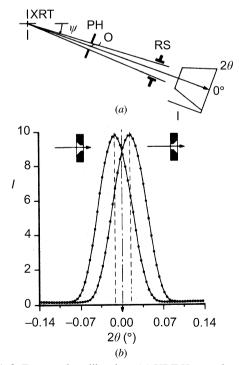
Fig. 2.3.1.6. Zero-angle calibration. (a) XRT X-ray tube anode,  $\psi$  takeoff angle, O axis of rotation, PH pinhole, RS receiving slit. Intensity distribution at right. (b) 0° position is median of two curves recorded with 180° rotation of PH.
