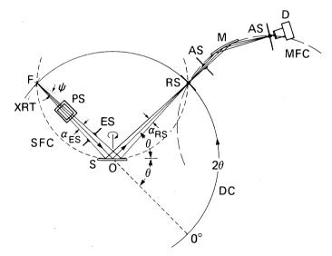
Fig. 2.3.1.3. X-ray optics in the focusing plane of a 'conventional' diffractometer with reflection specimen, diffracted-beam monochromator, and  $\theta$ -2 $\theta$  scanning:  $\psi$  take-off angle, DC diffractometer circle, MFC monochromator focusing circle,  $\alpha_{\rm ES}$  and  $\alpha_{\rm RS}$  entrance- and receiving-slit apertures,  $\theta$  Bragg angle,  $2\theta$  reflection angle, *O* diffractometer and specimen rotation axis; other symbols listed in Fig. 2.3.1.1.
