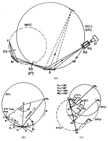
Fig. 2.3.1.13. Seemann–Bohlin method. (a) X-ray optics using incidentbeam monochromator. (b) X-ray tube line-focus source showing geometrical relations:  $\gamma$  mean angle of incident beam,  $\beta_H$  inclination of reflecting plane H to specimen surface,  $\theta_H$  Bragg angle of H plane, t tangent to focusing circle at O. (c) Diffractometer settings for various angular ranges.
