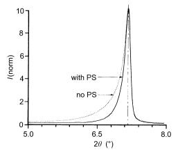
Fig. 2.3.1.11. Effect of axial divergence on profile shape. Narrow profile recorded with parallel slits (PS),  $\delta = 4.4^{\circ}$  between monochromator and detector Fig. (2.3.1.12), and broad profile with these parallel slits removed. Faujasite, Cu  $K\alpha$ ,  $\alpha_{\rm ES}$  2°.
