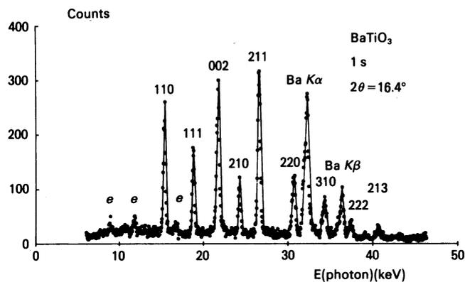
Fig. 2.5.1.2. XED powder spectrum of  $\text{BaTiO}_3$  recorded with synchrotron radiation from the electron storage ring DORIS at DESY-HASYLAB in Hamburg, Germany. Counting time 1 s. Escape peaks due to the Ge detector are denoted by  $e$  (from Buras, Gerward, Glazer, Hidaka & Olsen, 1979).
