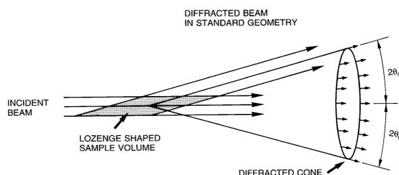
Fig. 2.5.1.1. Standard and conical diffraction geometries:  $2\theta_0 =$  fixed scattering angle. At low scattering angles, the lozenge-shaped sample volume is very long compared with the beam cross sections (after Häusermann, 1992).
