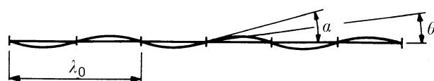
Fig. 4.2.1.8. Electron trajectory within a multipole wiggler or undulator. \lambda_0 is the spatial period, \alpha the maximum deflection angle, and \theta the observation angle. From Buras & Tazzari (1984); courtesy of ESRP.
