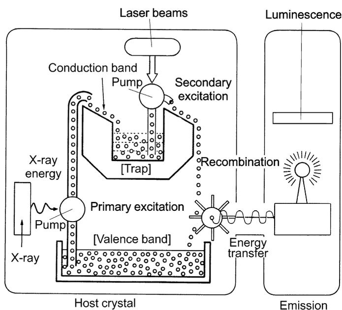
Fig. 7.1.8.1. Mechanism of photo-stimulated luminescence.
