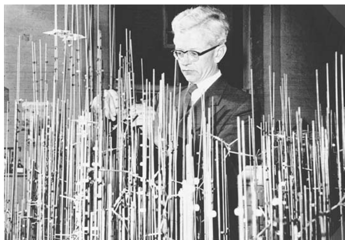
Fig. 1.2.6.1. The 2 Å-resolution map of sperm-whale myoglobin was represented by coloured Meccano-set clips on a forest of vertical rods. Each clip was at a grid point. The colour of the clip indicated the height of the electron density. The density was interpreted in terms of 'Corey-Pauling' models on a scale of 5 cm = 1 Å. Pictured is John Kendrew. (This figure was provided by M. F. Perutz.)
