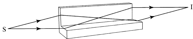
Fig. 6.1.4.2. The 'catamegonic' arrangement of Montel (1957), in which two confocal mirrors with orthogonal curvatures lie side-by-side.
