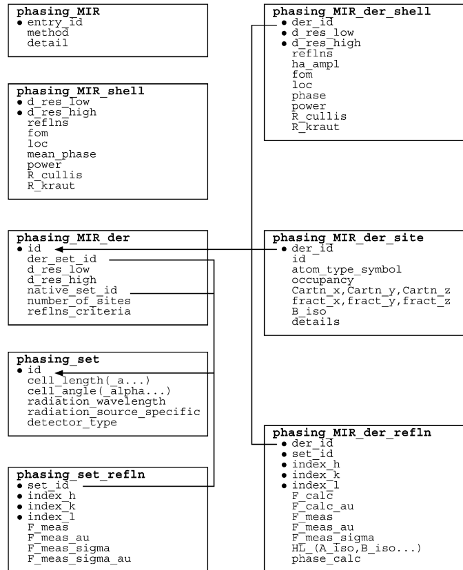
Fig. 3.6.6.2. The family of categories used to describe MIR phasing. Boxes surround categories of related data items. Data items that serve as category keys are preceded by a bullet (•). Lines show relationships between linked data items in different categories with arrows pointing at the parent data items.
