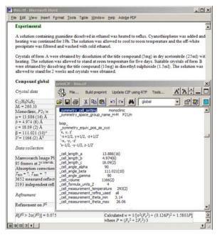
Fig. 5.3.3.13. The dual RTF/CIF editing windows in the *printCIF for Word* application. In this example, the author has selected the word 'Monoclinic' in the read-only table of crystal data; the corresponding CIF data item \_symmetry\_cell\_setting is highlighted in the CIF window, where it may be edited.
