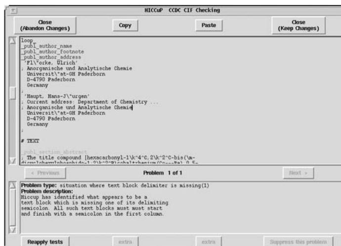
Fig. 5.3.3.9. *HICCuP* edit window and error description.
