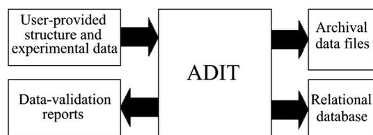
Fig. 5.5.3.1. Functional diagram of the *ADIT* system.
